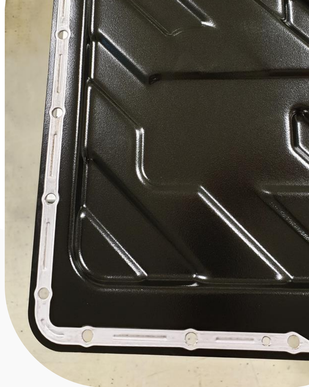
Selective paint stripping on a cathodic dip coated cover for battery trays
